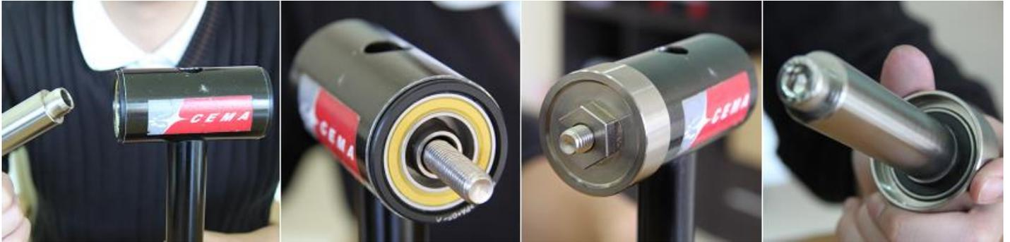
**Step 2. Place the removal ring(24mm, PN: SRC-TT-B006C-08) then insert the extractor tube through the Drive side bearing, lock the external cup, and tighten the screw to remove the bearing.**
