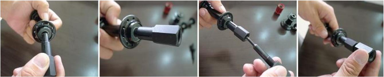
**Step 3. Screw puller handle into bearing puller and slide handle weight sharply downwards to remove bearing.**
