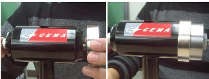
**Step 5. Tighten the screw to remove the BB set. Repeat the same process for another one.**
