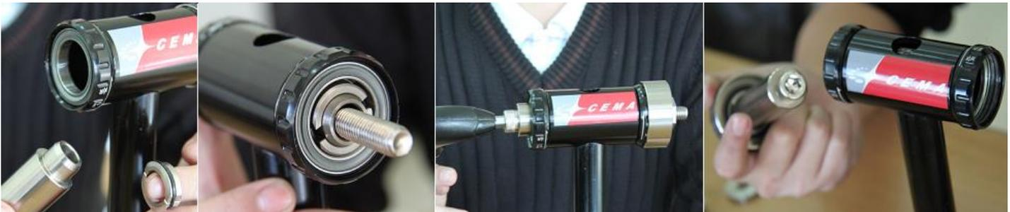
**Step 3. CEMA Bearing Kit. Place the spacer first, CEMA bearing (SRC-BB-S004 / SRC-BB-S006) onto the adapter (22mm) and fit bearing cup.**
