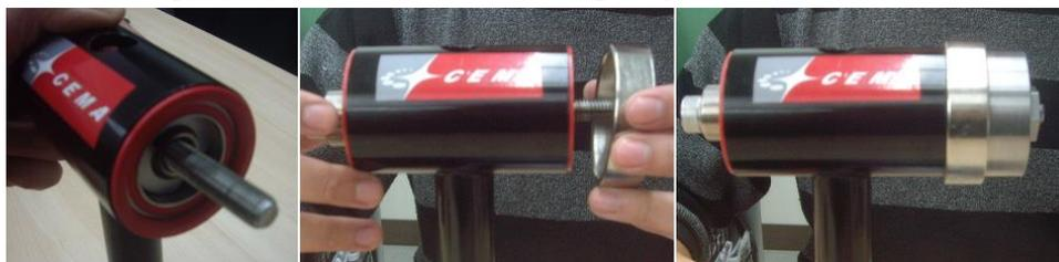
**Step 5. Tighten to remove BB cup, repeat process for the other cup.**
