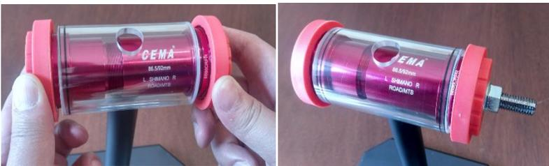
**Step 3. Tighten up the bottom bracket to the bottom bracket shell until there is no gap between the bracket and the shell.**
