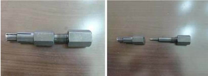
**Step2. Push bearing puller into bearing and tighten.**
