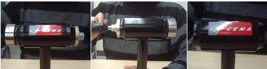
**Step 3. Insert the extractor tube with the removal ring (30mm, PN: SRC-TT-B006C-09) through the frame to the bearing.**
