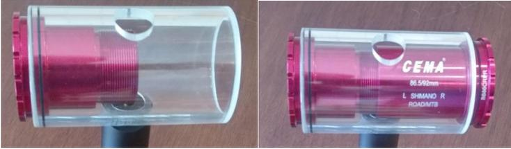
**Step 2. Insert the bottom bracket adapter (SRC-TT-B014/B015) and tighten the thread screw.**
