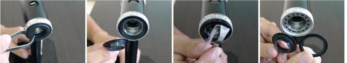
Step 2. Place bearing removal ring (OD24mm,PN: SRC-TT-B006C-08) on extractor tube, then put through the frame.
