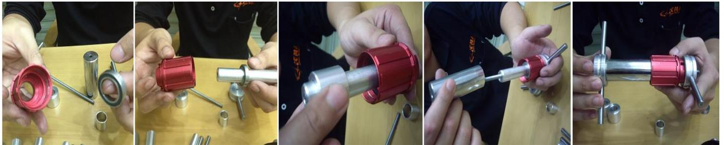
**Step2.** Use the same process to fit the second bearing.
