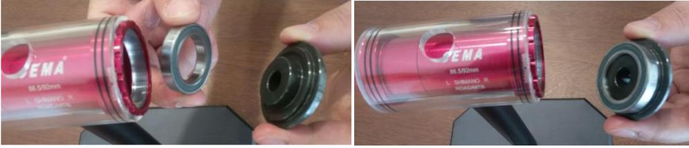
**Step 2. Insert the screw to the new bearing with the adapter then insert it through the bottom bracket. Install the bearing cup on the other side of the screw.**
