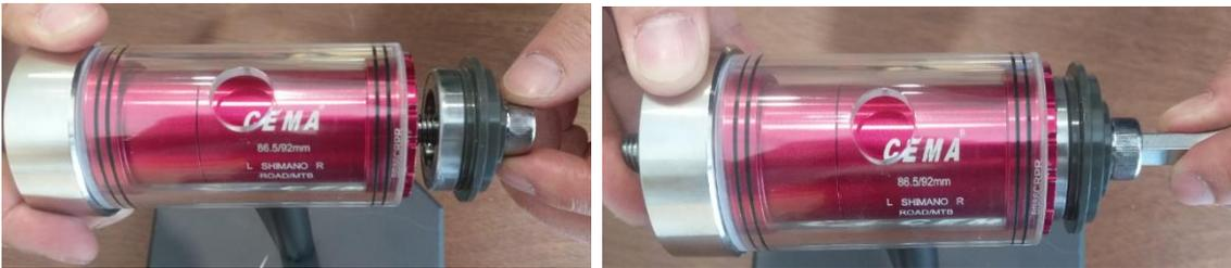
**Step 3. Tighten up the screw to fit the bearing. Then remove the screw and the adapter.**
