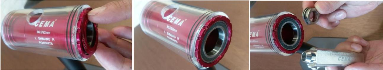
**Step 2. Insert the thread screw through extractor tube then lock the external bearing cup.**
