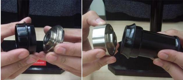
**Step 2. Place both side tightly to the frame, and tighten the screw to install the bearing set into the frame.**
