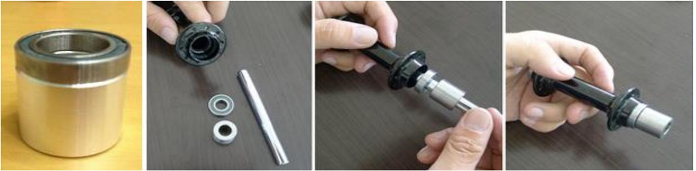
**Step2.** Insert threaded screw and external bearing adapter thread on tightening bars and tighten to fit bearings.
