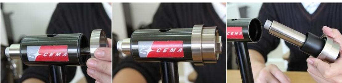
**Step 5. Insert screw BB spacer and add spacer (PF86 / 92) then thread on bearing cup into the tube, tighten the external bearing cup to remove the BB set.**
