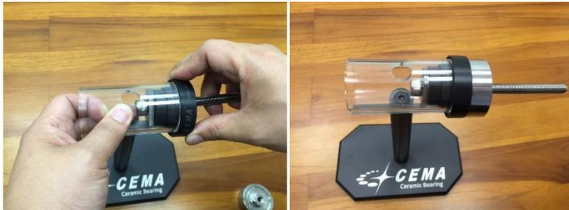
**Step 3. Press-fit the thread screw and roll hex wrench while making sure that the rim of the hand adapter stays parallel to the rim of the external bearing cup.**
