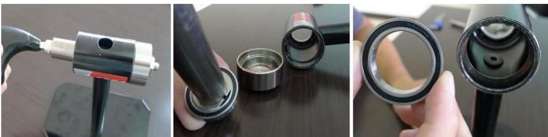
**Step 3. CEMA Bearing Kit. Place CEMA bearing (SRC-BB-BC30 / SRC-BB-BS30) onto the adapter (30mm) and fit the frame, place the adapter on another side to place correctly.**
