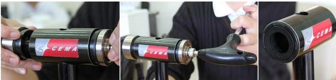
**Step 3. Place the removal ring (24mm, PN:SRC-TT-B006C-08) onto the extractor tube and insert into BB.**
