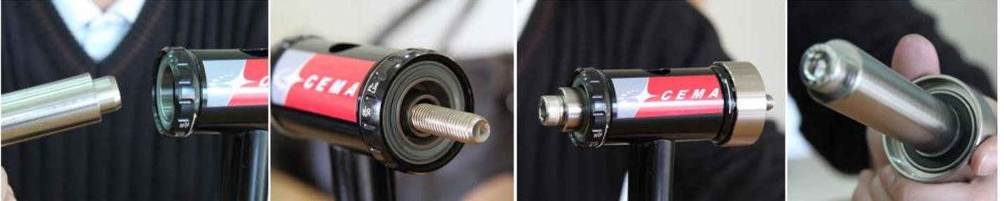
**Step 2. Place the removal ring(24mm PN: SRC-TT-B006C-08,) then insert the extractor tube through the Drive side bearing, lock the external cup, and tighten the screw to remove the bearing.**
