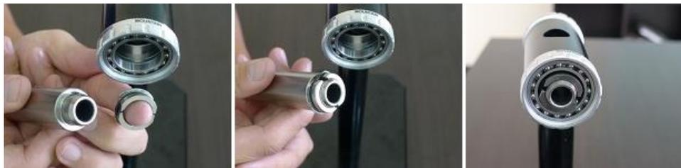
Step 3. Insert thread screw and fit bearing cup. Tighten screw to remove bearing.
