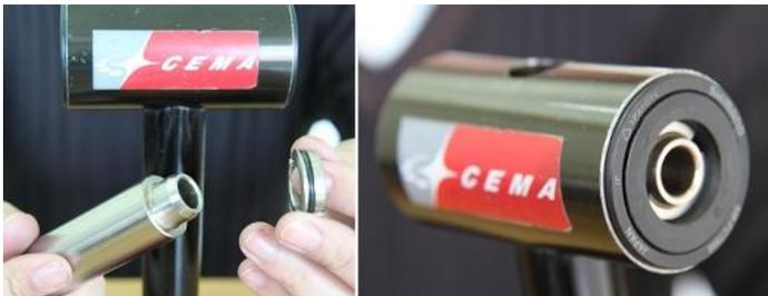
**Step 4. Insert screw add spacer (PF86 / 92) and thread on bearing cup into the tube then tighten the external bearing cup.**
