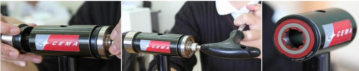
**Step 3. Remove the bearings from the frame, and insert the extractor with the removal ring(30mm) into frame.**
