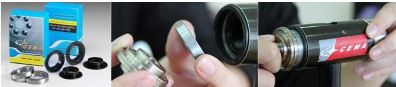
Step 5. Tighten screw to fit bearing and then replace caps.
