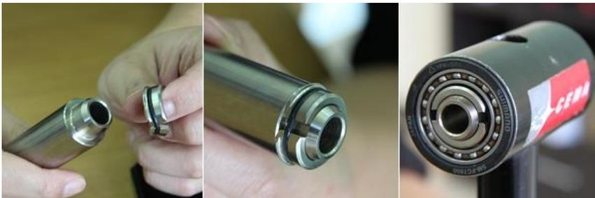
Step 3. Fit bearing cup, tighten screw to remove bearing, remove another one with the same way.
