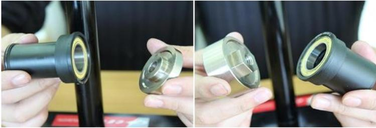
**Step 2. Place both side tightly to the frame, and tighten the screw to install the bearing set into the frame.**
