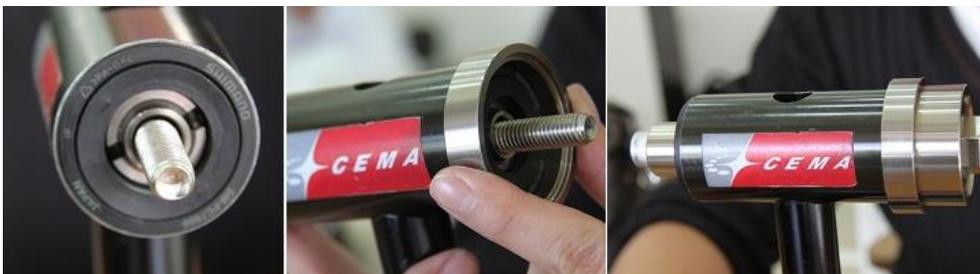
**Step 5. Tighten to remove BB cup, repeat process for the other cup.**
