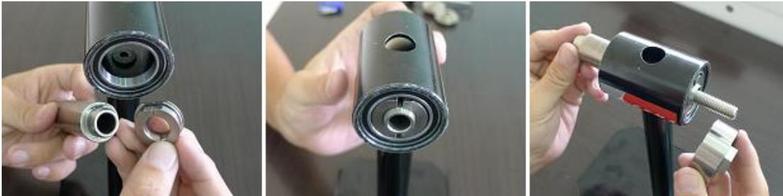
**Step 2. Tighten the screw to remove the bearing, repeat process for the other one.**
