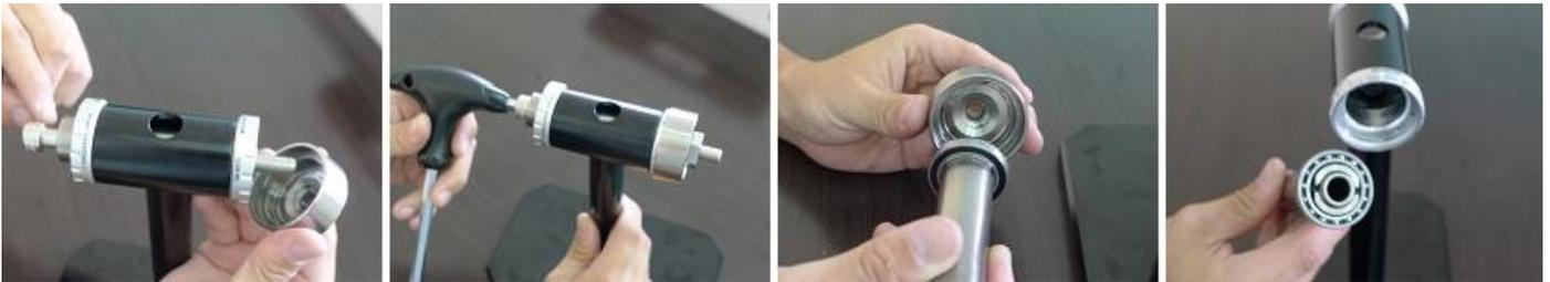
Step 4. CEMA Bearing Kit. Place CEMA bearing (SRC-BB-S003 / SRC-BB-S005) onto adapter and fit bearing cup (OD25mm).
