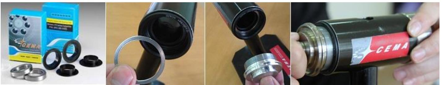
**Step 4. Tighten screw to fit bearing and then replace caps.**
