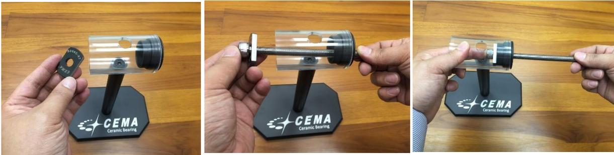
**Step 2. Insert the thread screw into the spacer (BB86/PF30/386) and the external bearing cup. Then lock the external bearing cup.**
