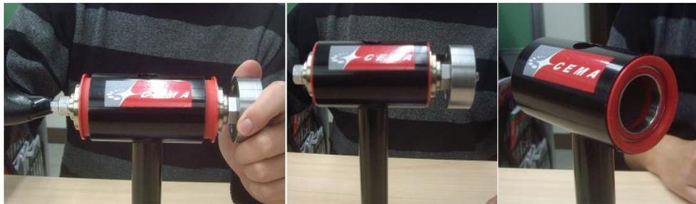
**Step 3. Place the removal ring (30mm) onto the extractor tube and insert into BB.**
