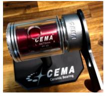
Step 3. Use cups to hold 2 sides and fasten up to 40~50NM
