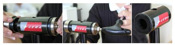
Step 3. Place the removal ring (24mm, PN:SRC-TT-B006C-08) onto the extractor tube and insert into BB.
