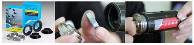
Step 5. Tighten screw to fit bearing and then replace caps.
