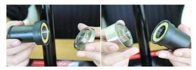
Step 2. Place both side tightly to the frame, and tighten the screw to install the bearing set into the frame.
