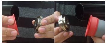
Step 2. Place both side tightly to the frame, fit the external bearing cup and tighten the screw to install the bearing set into the frame.
