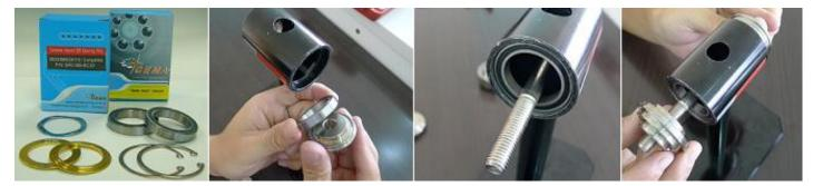
Step 4. Tighten cup and screw to fit bearing and then replace caps. Repeat the process for the other one.
