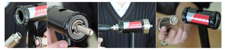
Step 3. CEMA Bearing Kit. Place the spacer first, CEMA bearing (SRC-BB-S004 / SRC-BB-S006) onto the adapter (22mm) and fit bearing cup.
