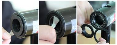
Step 2. Place bearing removal ring (OD24mm, PN: SRC-TT-B006C-08) on extractor tube, then put through the frame.
