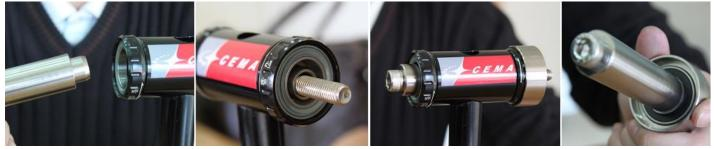
Step 2. Place the removal ring(24mm PN: SRC-TT-B006C-08,) then insert the extractor tube through the Drive side bearing, lock the external cup, and tighten the screw to remove the bearing.
