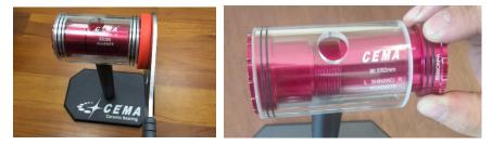
Step 2. Insert the thread screw into the external bearing cup.
