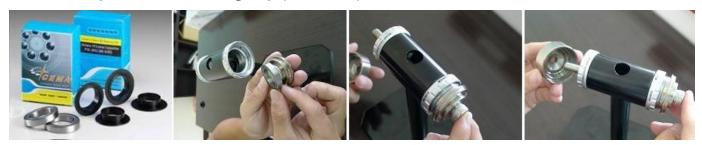
Step 5. Tighten screw to fit bearing and then replace caps.
