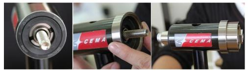
Step 5. Tighten to remove BB cup, repeat process for the other cup.
