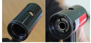
Step 4. Insert screw add spacer (PF86 / 92) and thread on bearing cup into the tube then tighten the external bearing cup to remove the BB set.
