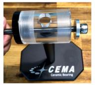
Step 3. Use SRC-TT-B006D-16 and fasten SRC-TT-B006-14(screw) with Allen key
