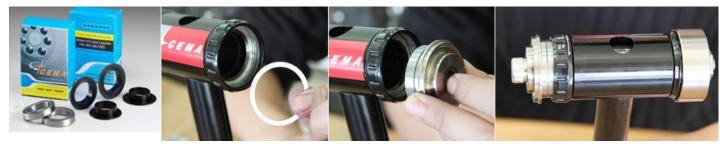
Step 4. Tighten screw to fit bearing and then replace caps.
