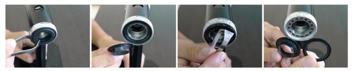
Step 2. Place bearing removal ring (OD24mm,PN: SRC-TT-B006C-08) on extractor tube, then put through the frame.
