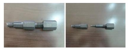
Step2. Push bearing puller into bearing and tighten.
