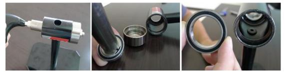
Step 3. CEMA Bearing Kit. Place CEMA bearing (SRC-BB-BC30 / SRC-BB-BS30) onto the adapter (30mm) and fit the frame, place the adapter on another side to place correctly.
