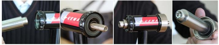
Step 2. Place the removal ring(24mm PN: SRC-TT-B006D-08) then insert the extractor tube through the Drive side bearing, lock the external cup, and tighten the screw to remove the bearing.
