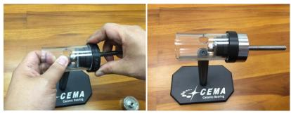
Step 3. Press-fit the thread screw and roll hex wrench while making sure that the rim of the hand adapter stays parallel to the rim of the external bearing cup.
