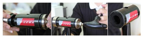
Step 3. Place the removal ring (24mm, PN:SRC-TT-B006D-08) onto the extractor tube and insert into BB.
