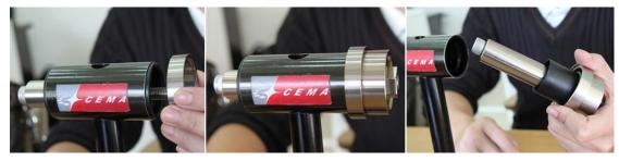
Step 5. Insert screw BB spacer and add spacer (PF86 / 92) then thread on bearing cup into the tube, tighten the external bearing cup to remove the BB set.
