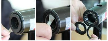
Step 2. Place bearing removal ring (OD24mm, PN: SRC-TT-B006D-08) on extractor tube, then put through the frame.
