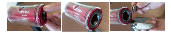
Step 2. Insert the thread screw through extractor tube then lock the external bearing cup.
