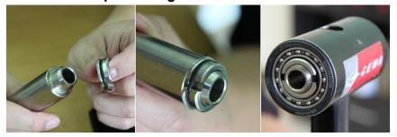
Step 3. Fit bearing cup, tighten screw to remove bearing, remove another one with the same way.
