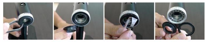
Step 2. Place bearing removal ring (OD24mm, PN: SRC-TT-B006D-08) on extractor tube, then put through the frame.
