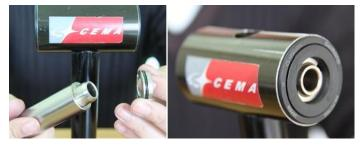
Step 4. Insert screw add spacer (PF86 / 92) and thread on bearing cup into the tube then tighten the external bearing cup.
