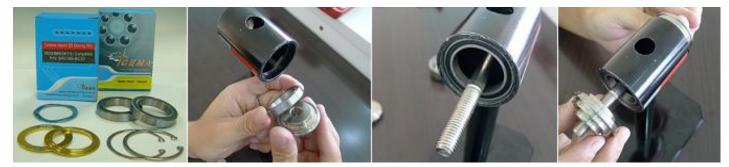
Step 4. Tighten cup and screw to fit bearing and then replace caps. Repeat the process for the other one.
