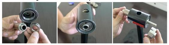
Step 2. Tighten the screw to remove the bearing, repeat process for the other one.
