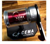
Step 3. Use cups to hold 2 sides and fasten up to 40~50NM
