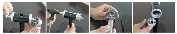
Step 4. CEMA Bearing Kit. Place CEMA bearing (SRC-BB-S003 / SRC-BB-S005) onto adapter and fit bearing cup (OD25mm).
