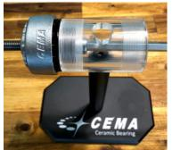
Step 4. Rotate with gasket and screw to remove the BB
