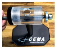
Step 3. Use SRC-TT-B006D-16 and fasten SRC-TT-B006-14(screw) with Allen key
